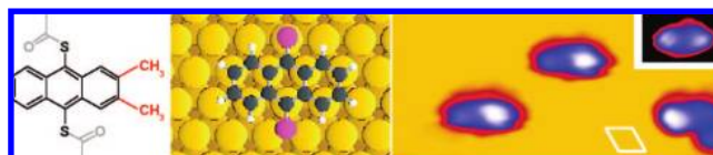
Figure 1. DMDTA (left) appears in STM ( 65 \times 30 \text{ \AA} , 1.4 V, 60 pA) with its long anthracene moiety and a unilateral protrusion reflecting the methyl substitution. For comparison, the insert shows an STM image of DTA.
